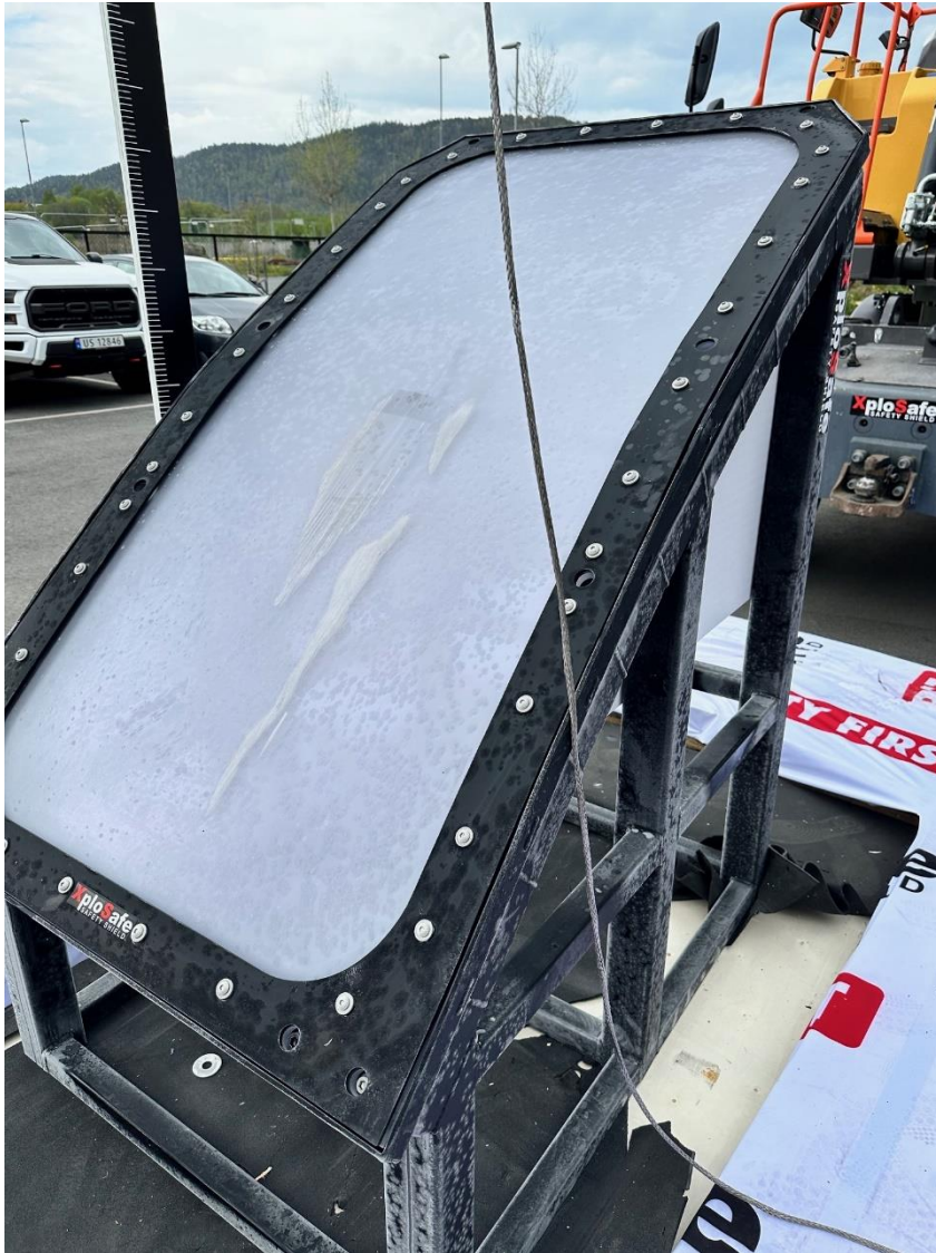
Picture 4. After drop test. No crack or broken glass. Only a slight dent and a few scratches
