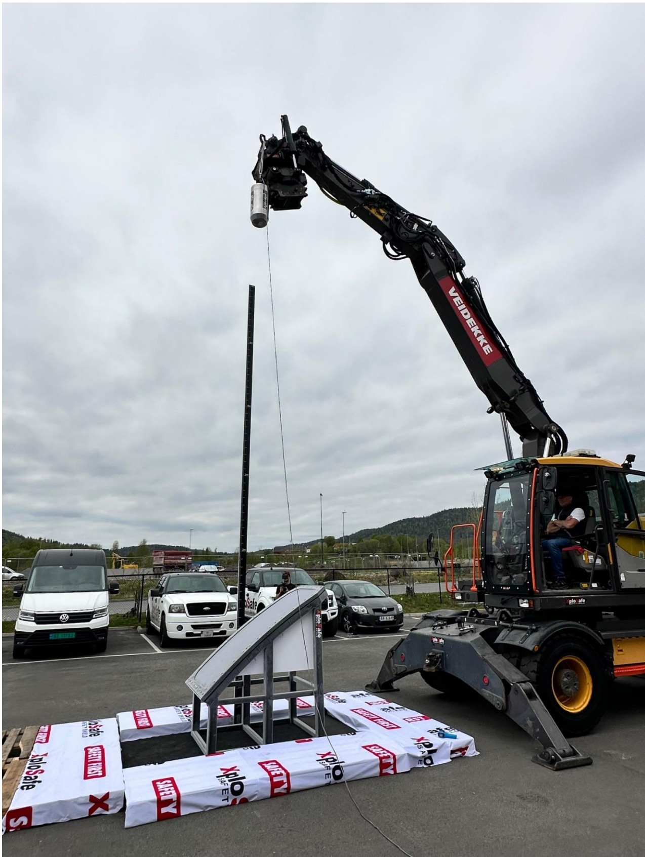
Picture 2. The test setup with drop of weights in free fall. The height of fall is 5.22 meters
