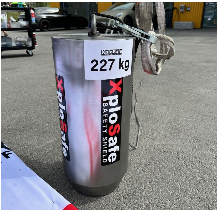
Picture 1. The door used weighs 227 kg and complies with ISO 3449
