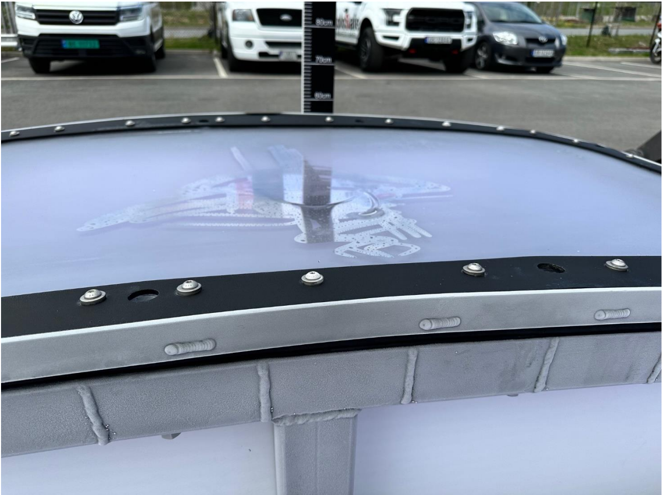
Picture 4. After drop test. No crack or broken glass. Only a slight dent and a few scratches
