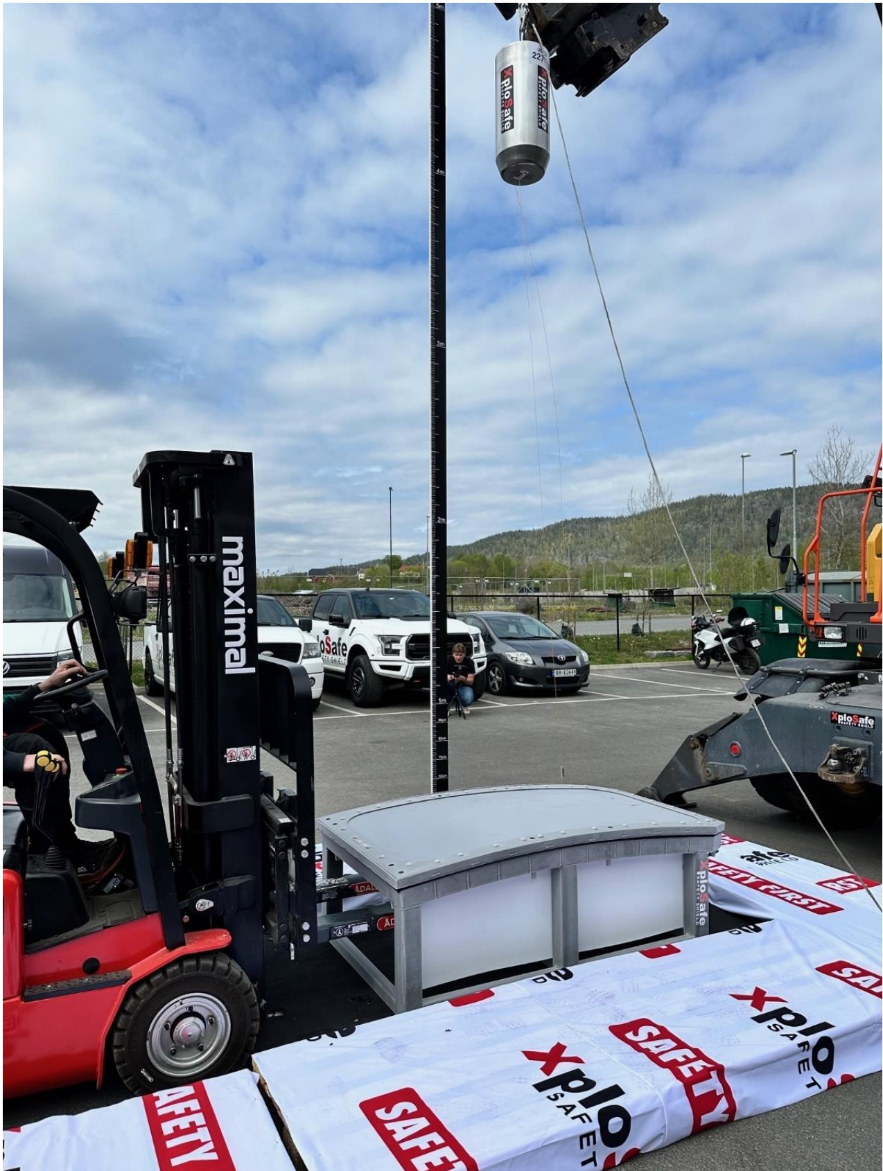
Picture 3. Just before the test. Drop height 2.61m and window has -18°C
