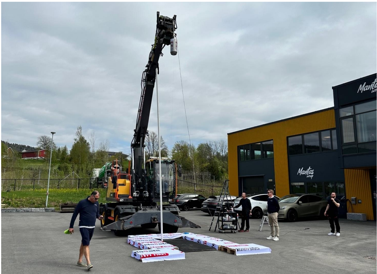
Picture 1. The free-fall drop weights test setup
