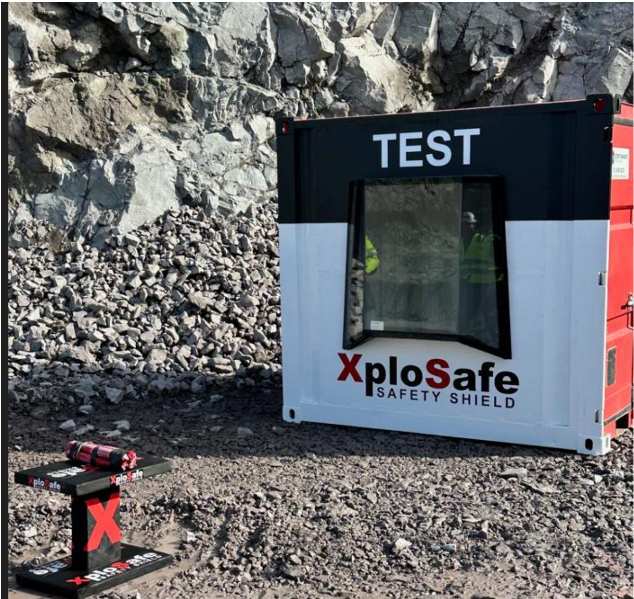
Image 2. 3 kg of dynamite placed 3 meters in front of the window with a height of 0.5 meters
