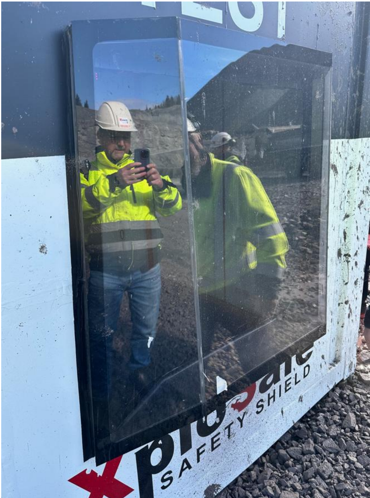
Image 5. After the explosion. The window is undamaged.
