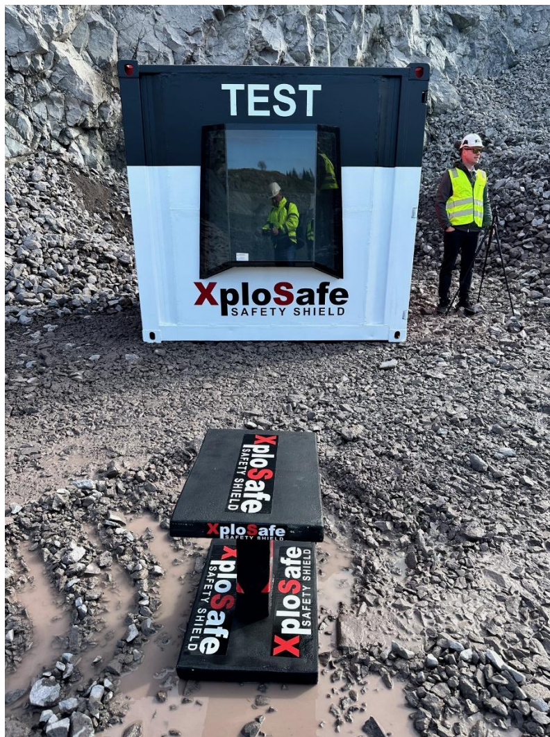
Image 1. Window made of polycarbonate mounted in a frame on an 8-foot container.
